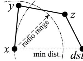
Fig. 2. Local minimum problem illustration:  $x$  faces the local minimum problem locating closer to  $dst$  than all its neighbors; as a result, it cannot forward packets further although a valid path through  $y$  exists
